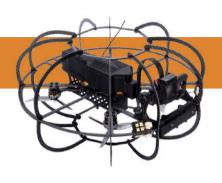
The aim of any inspection is to obtain the best possible set of data. To achieve this, the Stereo2 carries a 4k camera.
