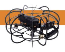
The Stereo2 is fitted with a lighting system specifically designed for inspections in confined spaces.
